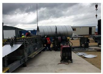
MOBILE PIPE can produce corrugated metal pipe in a variety of sizes
