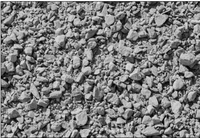
Dense Graded Aggregate (DGA).
