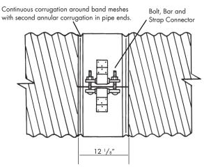
Standard construction is one-piece for 12" through 48", two-piece for 54" through 96", and three-piece for 102" and above.
