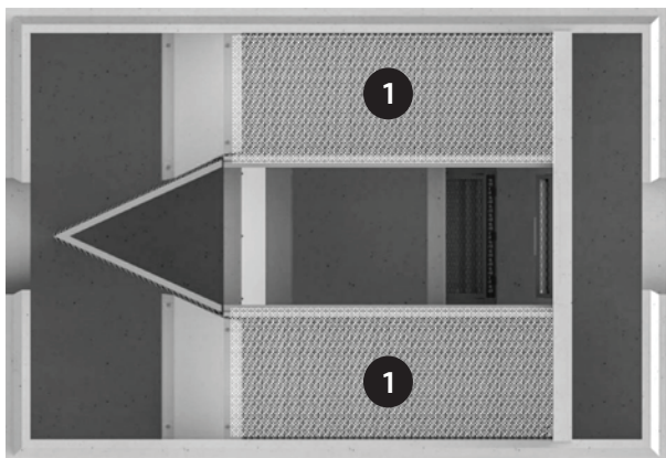
Top view into DSBB. Filtration screens (1) without sliding lids.
