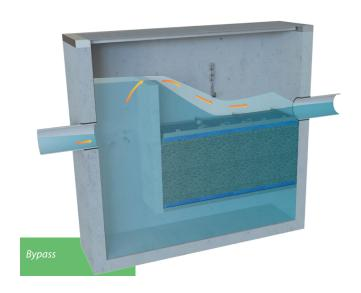
During peak flows, the internal weir allows water to bypass treatment eliminating the need for an external bypass or junction structure.
