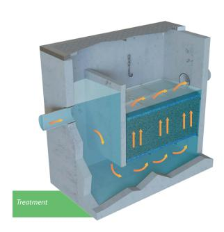
As water enters the system, head pressure builds behind the internal weir and sediment settles in the sump. Water then passes under the weir wall into the up-flow filter chamber. As water rises, it is forced through the media filtration bed for primary treatment before exiting the system.
