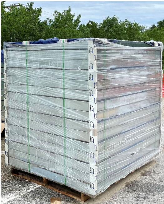
Forms are typically stacked on a pallet in heights up to 87" tall, but may vary project to project. The forms and pallet will be tightly bound for shipping and transport with shrink wrap and straps.
