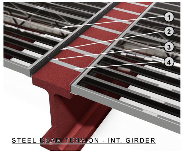
**1 – Structural Steel Joist, 2 – Steel Angle Support, 3 – Fillet Weld, 4 – Weld Anchor or Weld Strap**
