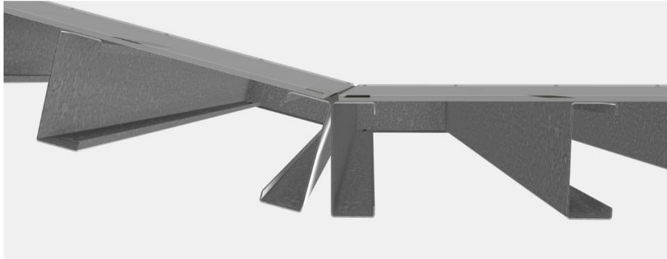
The longitudinal edge of the ClearCast form is then attached to the steel angle on the bridge beam with self-drilling screws prior to any loads being applied or the next form set.
