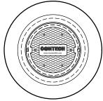
(SOLID CASTING) 30"Ø HS25 LOAD RATED 24"Ø HS20 LOAD RATED
