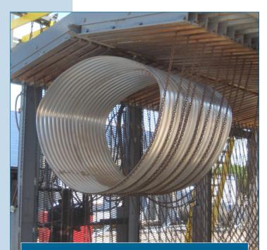
Large diameter Pipe-Arch manufactured in a chain arch press.
