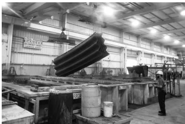
Black Steel MULTI-PLATE before the Zinc Tank
