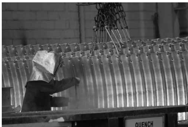
Galvanized MULTI-PLATE removed from the Zinc Tank
