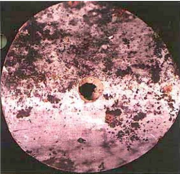
ALUMINIZED Type 2 - Invert - Waterside Mag. = 2X
