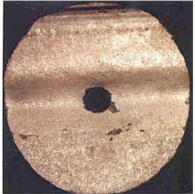
ALUMINIZED Type 2 Invert - Soilside
