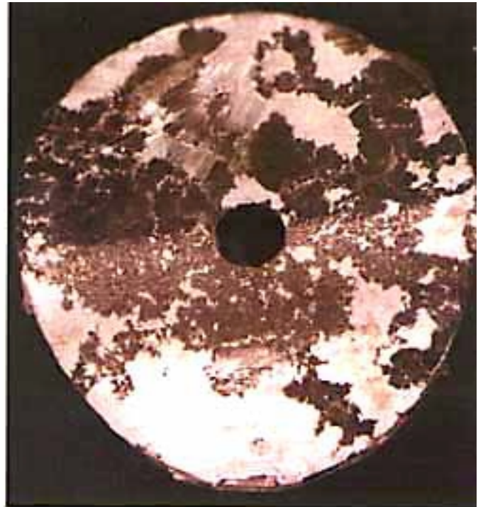
ALUMINIZED Type 2 Invert - Soilsid
