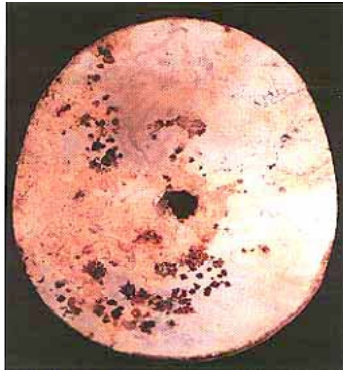
ALUMINIZED Type 2 - Invert - Soildside Mag. = 1.6X
