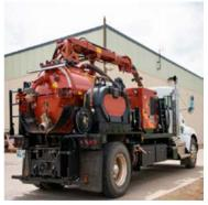
Vacuum Assisted Truck with Pressure Washer
