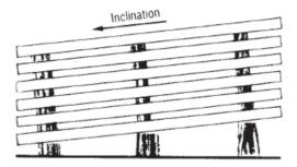
It should be noted that a wet storage stain results from the exposure conditions and is not indicative of inferior or poor quality galvanizing, or a degradation of the steel or aluminum.
