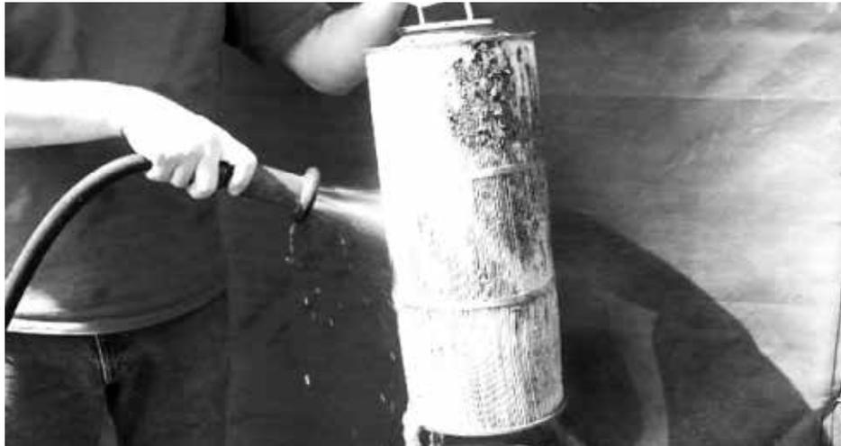
*4. To wash cartridges, remove from vault. Place over trash can and use a garden hose to spray clean.*
