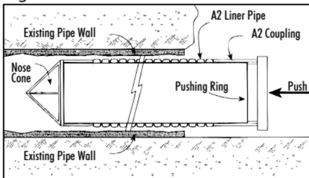
2. Both the gasket on the A2™ Liner spigot and the inside of the coupling should be lubricated prior to lowering the pipe into the existing (host) pipe and prior to joining. See the Assembling Gasketed Joints section on Page 13 for more information on joining pipe sections.
