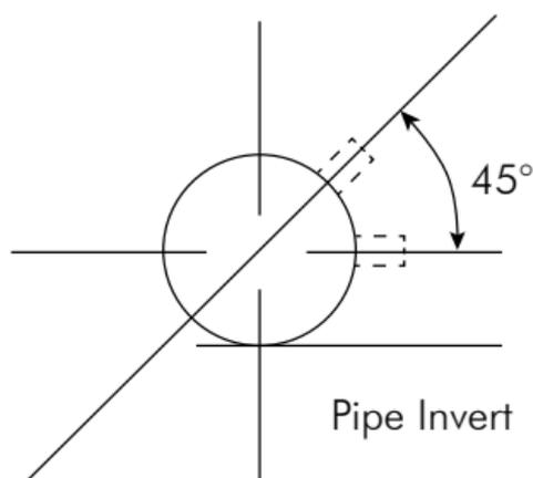
In order to minimize lateral pipe “punch-through” potential, it is recommended to install wye or tee fittings at an angle no greater than 45 degrees from the horizontal centerline. Stacks (saddle or other connection) at a 90 degree angle from the pipe’s horizontal centerline should not be allowed.
