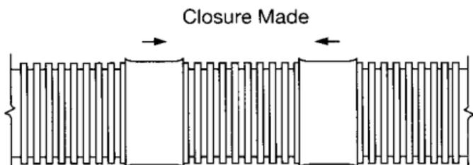
5. Align the measured length with terminal ends, and push closure couplings to homemarks. In addition to standard closure couplings, flexible rubber adapters, gasketed stainless steel clamps and manholes can also be used to connect terminal ends.
