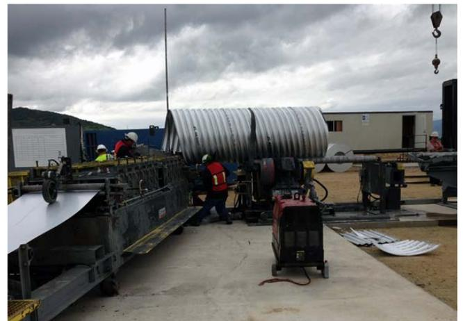
MOBILE PIPE can produce corrugated metal pipe in a variety of sizes
