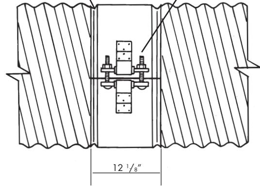
Standard construction is one-piece for 12" through 48", two-piece for 54" through 96", and three-piece for 102" and above.
