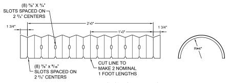
FIGURE 2. Standard Deck Drain Detail
