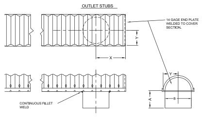
FIGURE 4. Deck Drain Outlet Stubs
