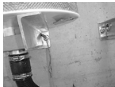
Figure 5. Cartridge clip in unlocked position (Maintenance)
