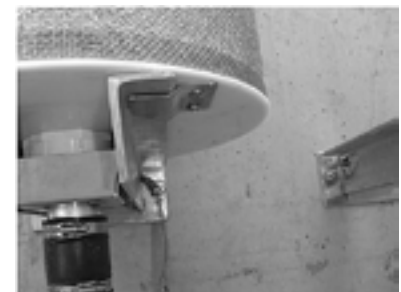
Figure 6. Cartridge clip in locked position (Operation)
