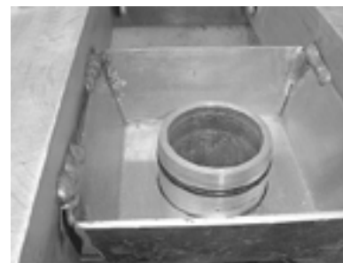
Figure 8. Single cartridge rack (hinge pin is inserted at the wall – remove to rotate rack into Up (Maintenance position)
