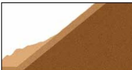
SHALLOW PLANE FAILURE
