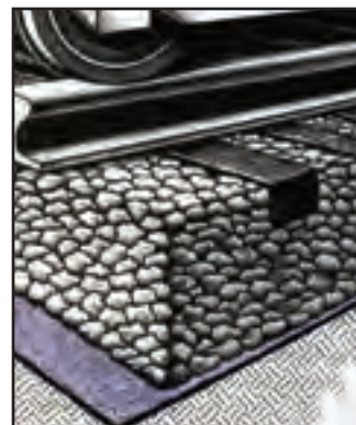
Robust Geotex® nonwovens stabilize subgrades and prevent the fouling of ballast beneath railway track.
