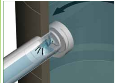
Fluidic-Amp Model Vortex Valve — typical for controlling small flows
