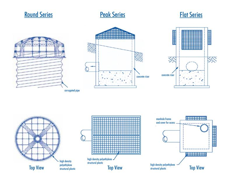
StormRax pyramid racks are available with an anti-vortex device and racks can be mounted on concrete structures, plastic and metal pipe.
