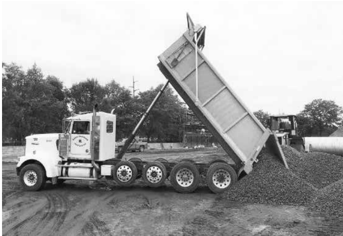
Examples of heavy construction equipment that may require additional minimal cover. Contech can help evaluate minimum cover for the installation contractor for all the equipment on the site.
