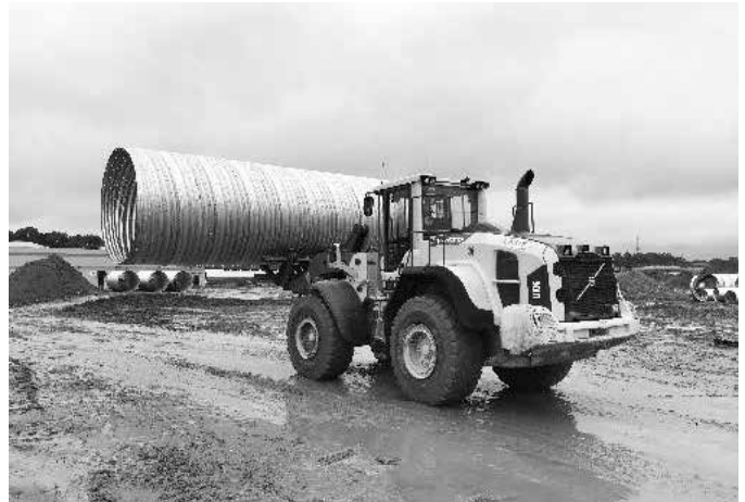
Examples of heavy construction equipment that may require additional minimal cover. Contech can help evaluate minimum cover for the installation contractor for all the equipment on the site.
