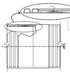
A2  $^{\text{\tiny TM}}$  Liner's patented STAB-JOINT coupler fits flush with the outer wall surface for easy insertion.
