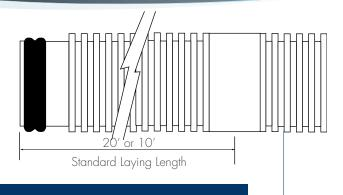
A2  $^{\text{\tiny TM}}$  Liner is available in standard lengths of 10 and 20 feet. 2.5-feet lengths are available for insertion via manholes.
