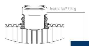
Either INSERTA TEE® or saddle tee fittings allow easy-to-make connections for  $A2^{TM}$  Liner. Saddle tee fittings employ stainless steel fasteners.
