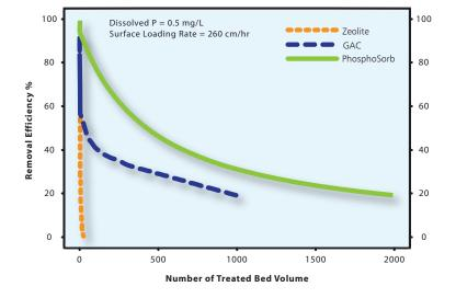
In laboratory testing, PhosphoSorb removed 50% of the first 1,000 treated empty bed volumes (EBVs) of 0.5 mg/L influent dissolved P solution, and lasted for at least 2,000 treated EBVs.
