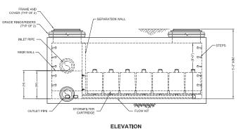
The Peak Diversion StormFilter is offered in 6 different sizes that are capable of handling up to 38 cartridges.
